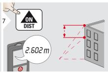
The result is shown in the main line and the measured distance above.
