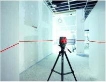
Pendulum based self-leveling The instrument is set up quickly thanks to a well-dampened pendulum, effortlessly projecting horizontal and vertical lines. Minor angular misalignments of 3.5°± 0.5° are compensated automatically. If the tilt is outside these limits, the laser lines will flash to prevent errors.
