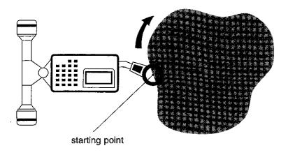
1. Put a mark at a point on the circumference of the drawing to be measured.
